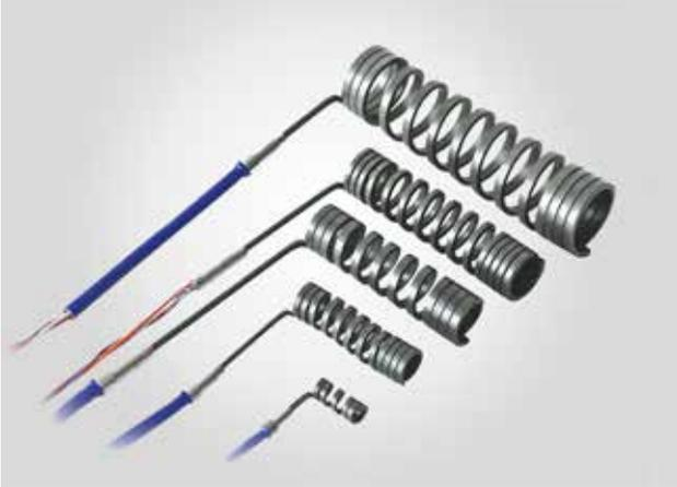
Coil Heaters are an advance concept of thermal engineering has a construction similar to high watt Coil Heaters are an advance concept of thermal engineering has a construction similar to high watt density cartridge heaters. These heaters are also known as high performance tubular heaters. The basic construction of these heaters consists of compacted MgO, high temperature resistance wire and chrome Nickel Steel Tube.
