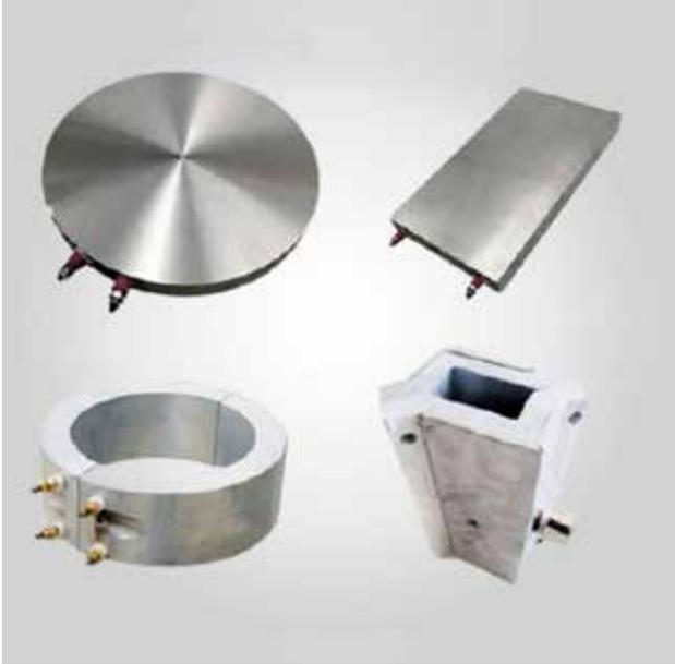
Cast-in heaters are designed for heating solids or indirect heating. Cast-in heating elements are ideal for applications requiring homogeneous indirect heat. Cast-in heaters are often used in plastics industry, packaging industry, food industry and many others. The cast-in heating plates and heating bands consist of one or several electrical resistance embedded in a block of aluminum, brass, bronze or cupronickel alloy.
